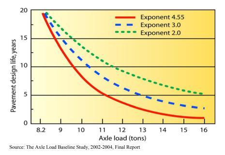
Figure 2 (adopted from SAxLS Figure 7.2.1 p 72) shows the difference between the produced ESALs when *payload increases on a given number of axles* and *when payload is constant and the number of axles carrying this payload decreases*. ESALs/tonnkm in
