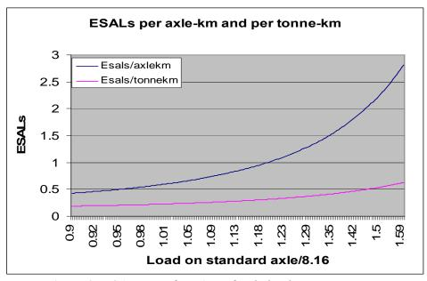
*Figure 2: ESALs as a function of axle loads* Source: Axle Load Study for Southern Africa (Fig. 7.2.1)
